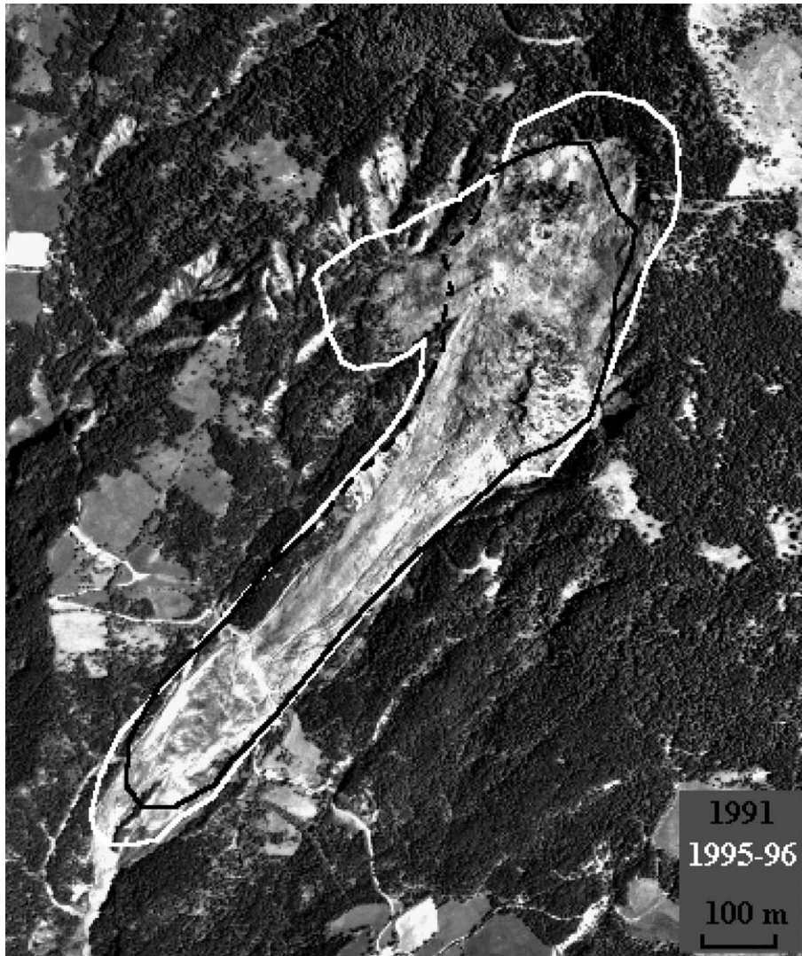
Fig. 10. Changes in the landslide boundaries between 1991 and 1996 deduced from SAR interferometry analysis marked on the aerial photograph.
